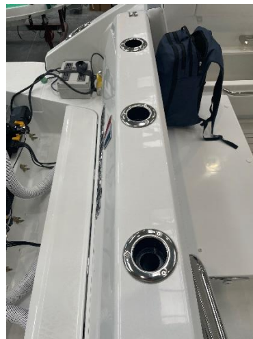
5 SST Rod Holders in aft cockpit bench backrest
